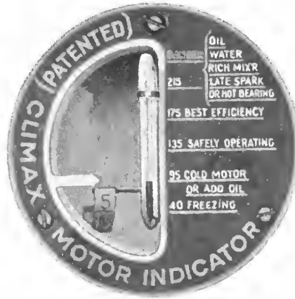
Climax motor indicator for dash mounting
